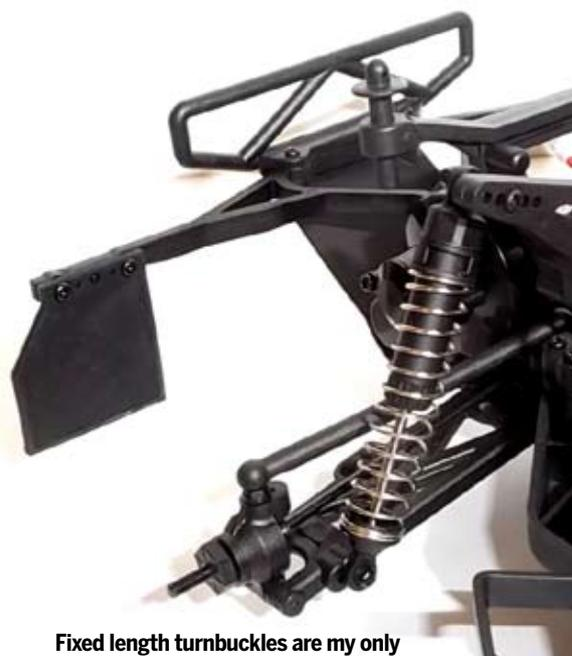
Fixed length turnbuckles are my only real criticism, I can even live with the clips to set shock pre-load
