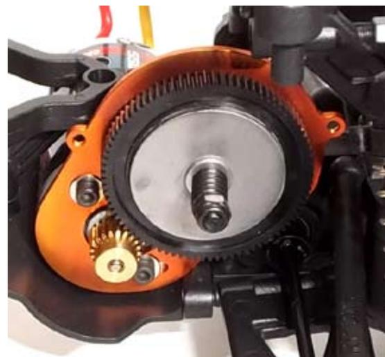
A twin plate slipper clutch is very much required. It allows you to help protect the driveline from damage
