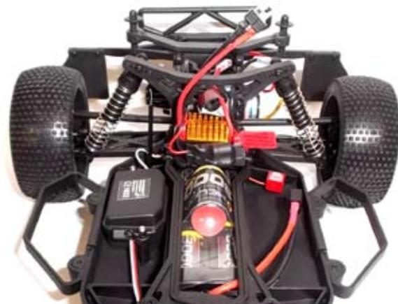
The layout is pretty well balanced, the receiver weighs next to nothing so won't upset handling even in that waterproof box
