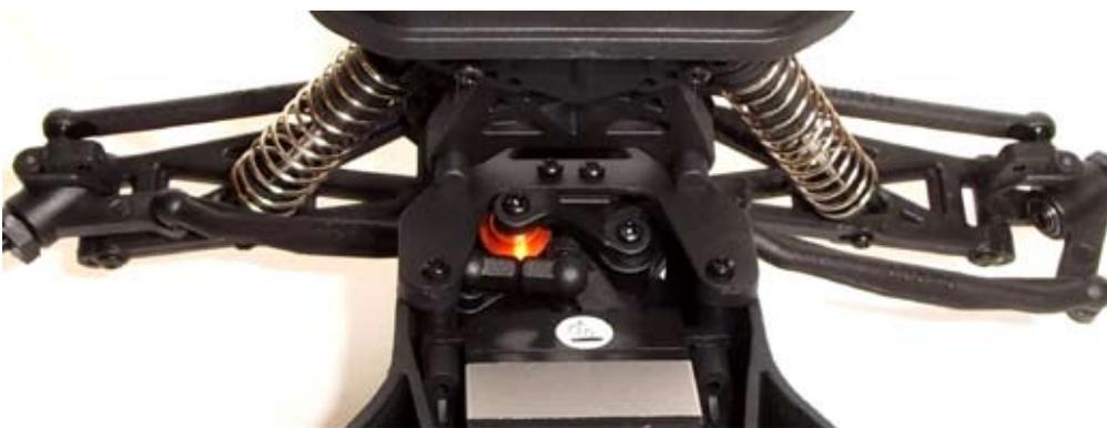
With a 6 kg steering servo and a very traditional bell-crank steering assembly, including adjustable servo saver - Helion have covered all the bases
