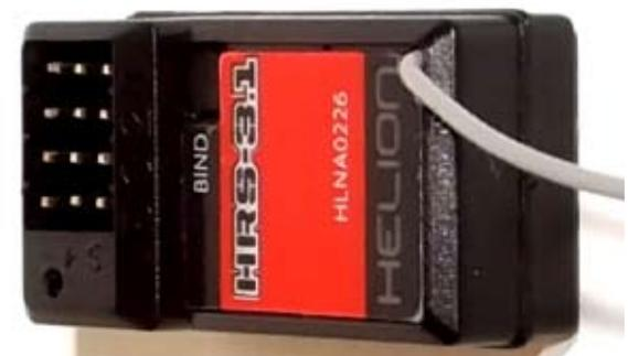
The tiny footprint Rx has a built-in bind button making the process of re-binding should you ever need to a simple affair
