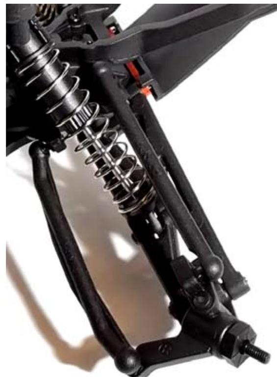
Again note the steering linkages, set length and solid plastic. No toe in or out options here
