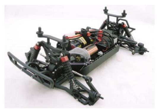
left of the chassis and feeds power into a spur gear which, worryingly, is not protected by a slipper clutch although the spur gear has the appropriate mouldings for a clutch setup.
