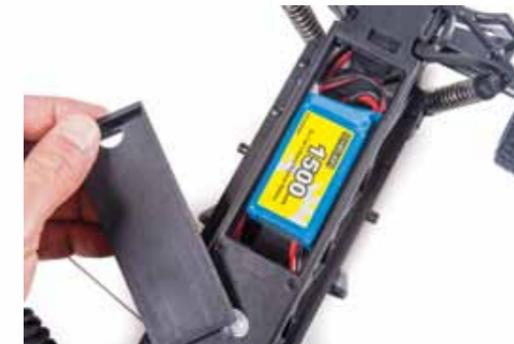
The supplied 2S LiPo battery pack is installed via a trap door in the chassis underside, and fits with room to spare.
