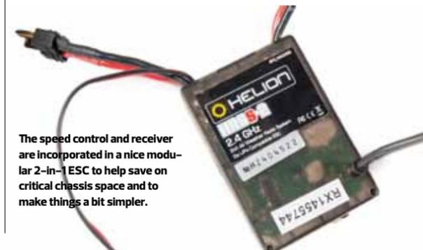
The speed control and receiver are incorporated in a nice modular 2-in-1 ESC to help save on critical chassis space and to make things a bit simpler.
