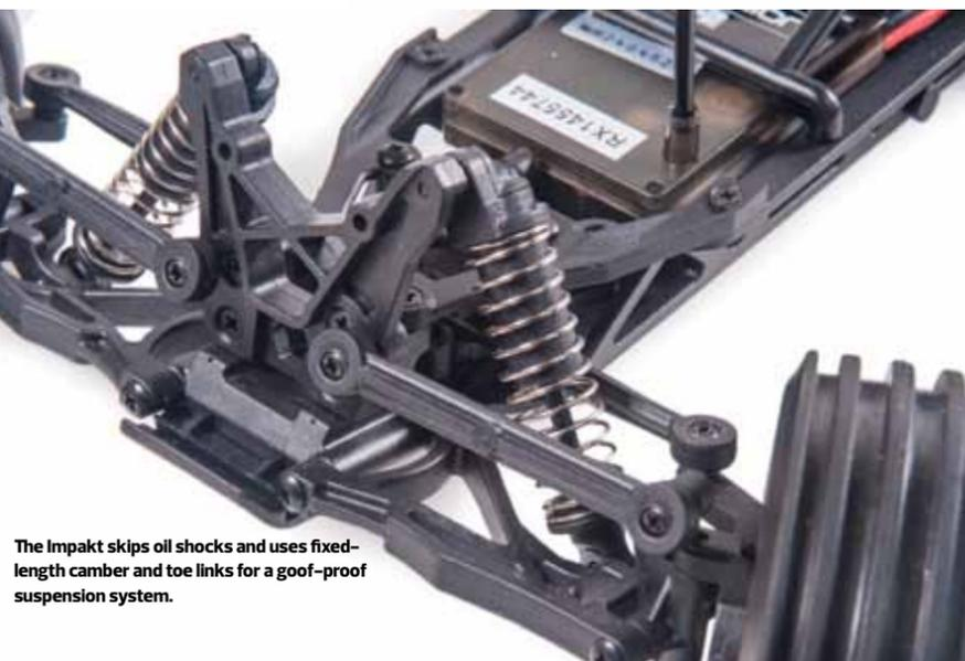
The Impakt skips oil shocks and uses fixed-length camber and toe links for a goof-proof suspension system.
