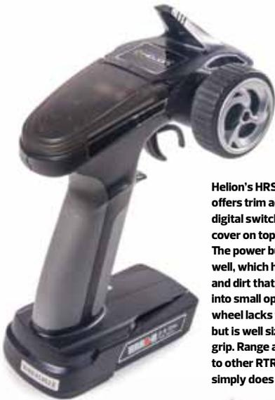
Helion's HRSS-2 2.4GHz radio offers trim adjustments only, via digital switches under a flip-up cover on top of the transmitter. The power button is under there as well, which helps to keep out dust and dirt that tends to find its way into small openings. The plastic wheel lacks foam for your fingers, but is well sized for control and grip. Range and feel are comparable to other RTR systems, the radio simply does its thing.
