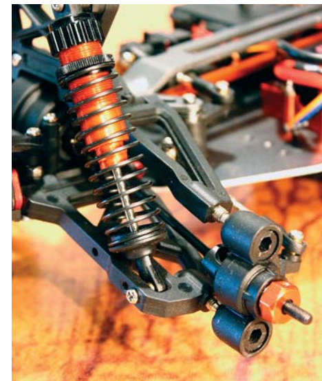
Left: The new rear hubs improve the durability of the Dominus and the clamping hex's are a big improvement over the stock units. Right: Up front, Helion's shocks offer ultra-smooth suspension damping and is a must have for any Dominus owner. The new universal axles are a highly recommended option too especially in the front.
