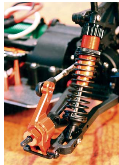
Left: The new rear hubs improve the durability of the Dominus and the clamping hex's are a big improvement over the stock units. Right: Up front, Helion's shocks offer ultra-smooth suspension damping and is a must have for any Dominus owner. The new universal axles are a highly recommended option too especially in the front.
