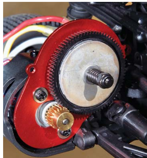
A dual pad slipper dampens the shock to the drivetrain. An aluminum motor plate helps dissipate heat from the motor as the buggy is geared to reach speeds over 30mph.
