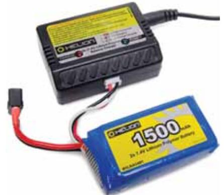
No upgrade required in the battery department, there's a LiPo right in the box. Helion supplies an AC-powered mini balance charger to juice it up, but its 0.5amp output requires about three hours to do the job. Expect about 15 minutes of run time per charge.
