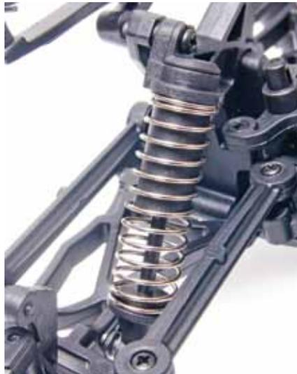
The plastic friction shocks do a good job of taming smaller obstacles, but are bouncy when the going gets rough.
