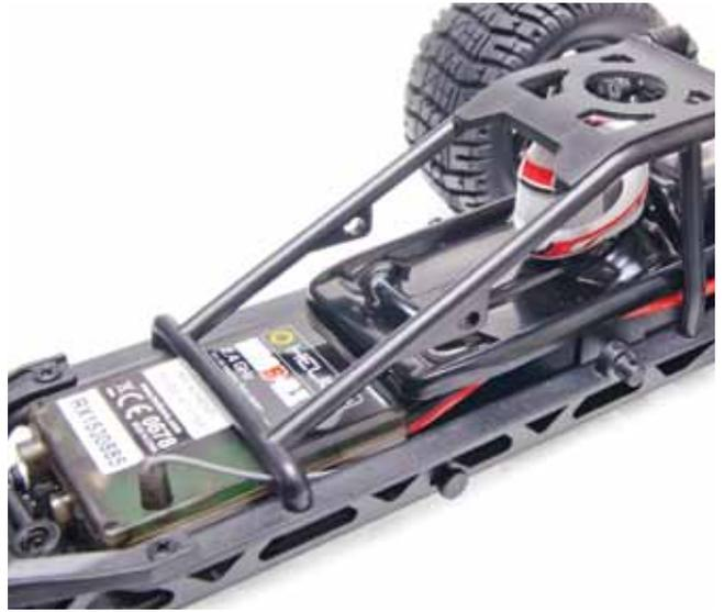
The speed control/receiver combo unit mounts ahead of the battery pack. The driver is hard to see with the body on, but he looks good under the roll cage.
