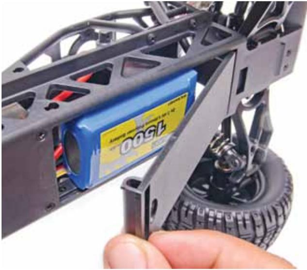
No body clips to remove here. The bottom loading battery compartment makes it easy to access the battery for quick removal and installation.
