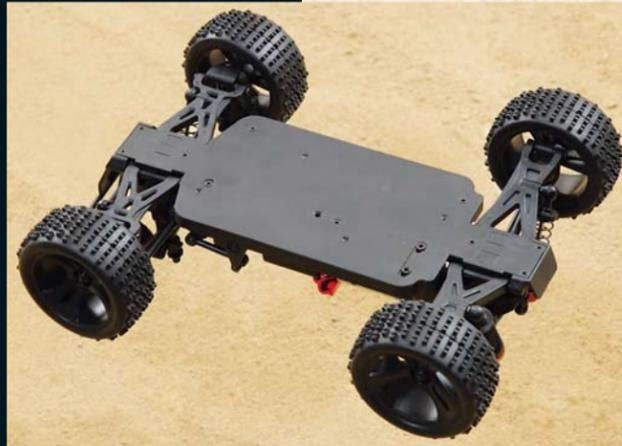
1/18 vehicles on the market. This means dirt and debris won't cut your fun short and ruin the spur gear. The Animus 18TR is also 4WD resulting in great traction and cornering speed. It features a light plastic drive shaft to deliver power to the front and rear of the vehicle. Both the front and rear differentials are of the gear variety and can be used for hours before requiring service
