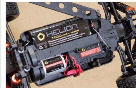
The motor and ERS unit are neatly positioned on the right hand side of the chassis while the battery sits on the left for a well-
