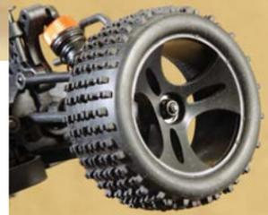
Aggressively treaded soft compound tires are mounted to cool looking black 3-spoke rims. The rims mount to the truck with miniature hex adapters so they run straight and true.
