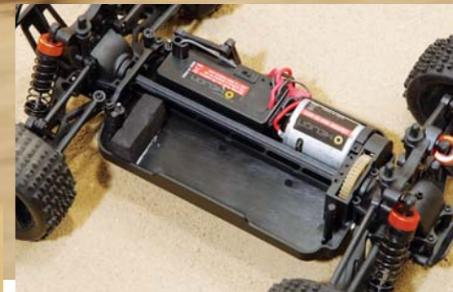
With the plastic top plate removed the lightweight plastic center driveshaft and spur gear are exposed on the Animus 18TR. The drivetrain is designed to keep all foreign objects out, reducing possible failure and maintenance.
