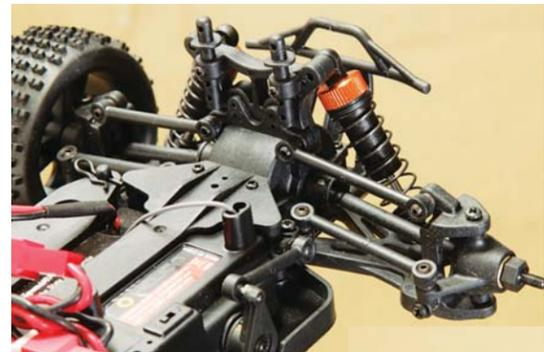
The front and rear suspension are typical of other 1/18 vehicles as they feature oil filled shocks, multiple mounting positions on the shock towers and fixed plastic turnbuckles. What really sets the Animus 18TR apart is the no slop steering linkage and spring loaded servo saver. This really helps the vehicle track straight.
