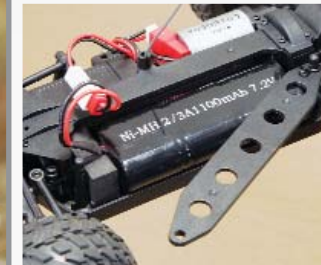
The battery compartment area is large enough to hold NiMH and LiPo batteries of various sizes and configurations so upgrading your pack is a non issue. The included foam spacer will help keep smaller sized packs in one place, and will allow you to position the pack to the front or rear of the chassis.
