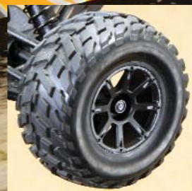
The compound terrain short course style tires are mounted to black 5-spoke rims. The rims mount to the truck with miniature hex adapters.
